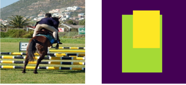
Figure 4. Example of weak segmentation ground-truth. Left: Input image with a size of 300 \times 300 , with a person and a horse. Right: Segmentation ground-truth for the left image, with a size of 38 \times 38 ; the pixels locate in both person and horse bounding-boxes will be assigned to person class since its bounding-box is smaller.
