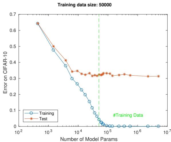
Fig. 3. Empirical and expected error in CIFAR 10 as a function of number of neurons in a 5-layer convolutional network. The expected classification error does not increase when increasing the number of parameters beyond the size of the training set.
