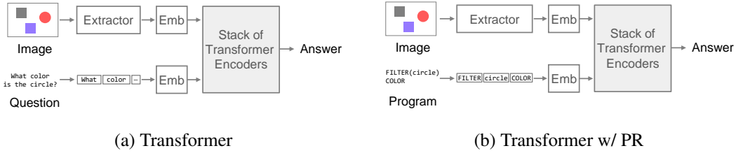
Figure 3: Transformer-based Baseline Methods . (a) Standard Transformer (Transformer) takes an image and a question as inputs. (b) Standard Transformer with programs (Transformer w/ PR) takes a program as an input instead of the question. Emb denotes visual/word embeddings. These approaches use the same visual inputs and Transformer encoder structure.
